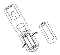
2 Insert two AA batteries into the battery compartment. Make sure the + and - symbols on the batteries align with the + and - symbols inside the battery compartment.
